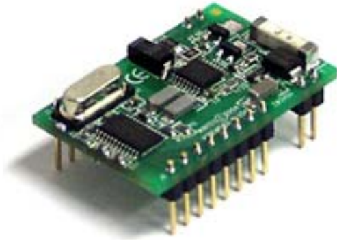
Figure 1: 24-pin DIP Package
